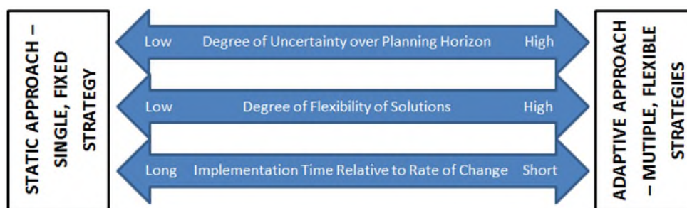
Figure 11 Conceptual representation of how to choose between static and adaptive approaches under uncertainty, Image reprinted from (Maier et al., 2016).
